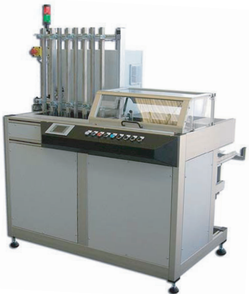
Modular bobbin magazine rack holds up to 40 empty bobbins and allows quick bobbin style changes.
